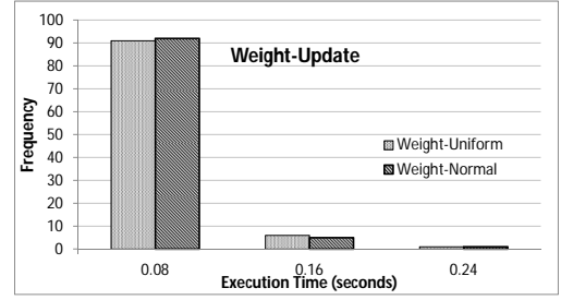
Figure 12: Distribution of the execution times of the Weight-Update operation on S_2 (uniform weight) and S_3 (normal weight)
