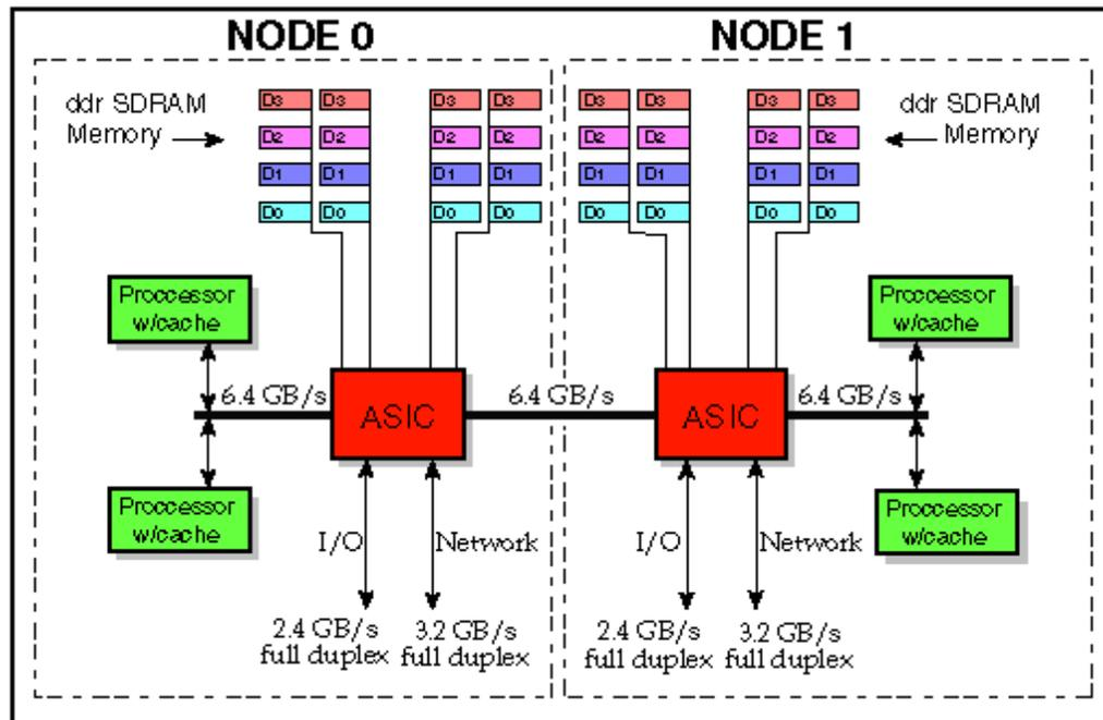
The NUMAflex allows to connect up to 512 processors, each can support 6.4 GB per second of bandwidth.
