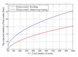
**Fig.2** The expected hop count between a random source and destination pair. The analysis results are compared with flooding and adaptive-gossiping according to question (5) in a given network size of  $(1000 \times 500)m^2$  with the total number of nodes from 60 to 1060.
