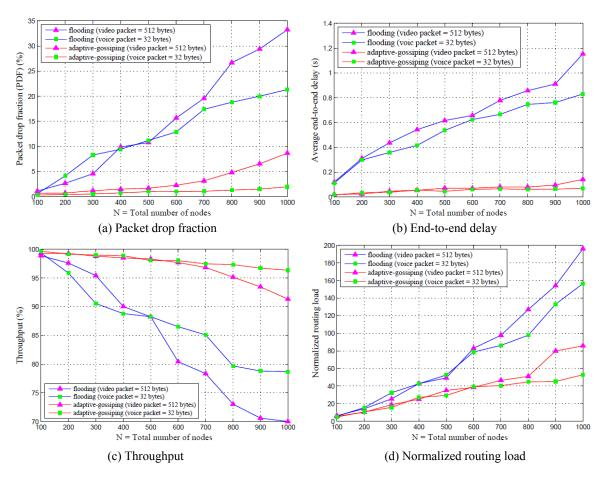
**Fig.4** The simulation results of multimedia communications with packet sizes of 32 and 512 bytes for voice and video data, respectively. The comparison of flooding and adaptive-gossiping is between 100 and 1000 nodes with 1 packet sent per second in a given network size of  $(1000 \times 500)m^2$ .
