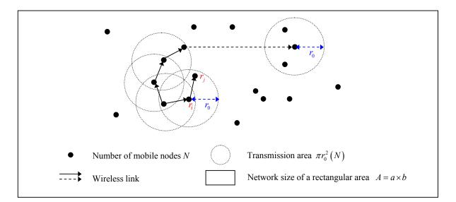
Fig.1 The model of network topology is an undirected random geometric graph. Nodes are randomly distributed in a network of size  $A=a \times b$  and each node has the same radio transmission range  $r_0$
